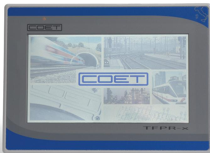
Multifunction digital Protective Relay combining measurements, control and protection for complete traction feeder management. It is suitable to be used in all the Traction systems like tramways, trolley bus, Metro and Railways Power Supply Substations.
