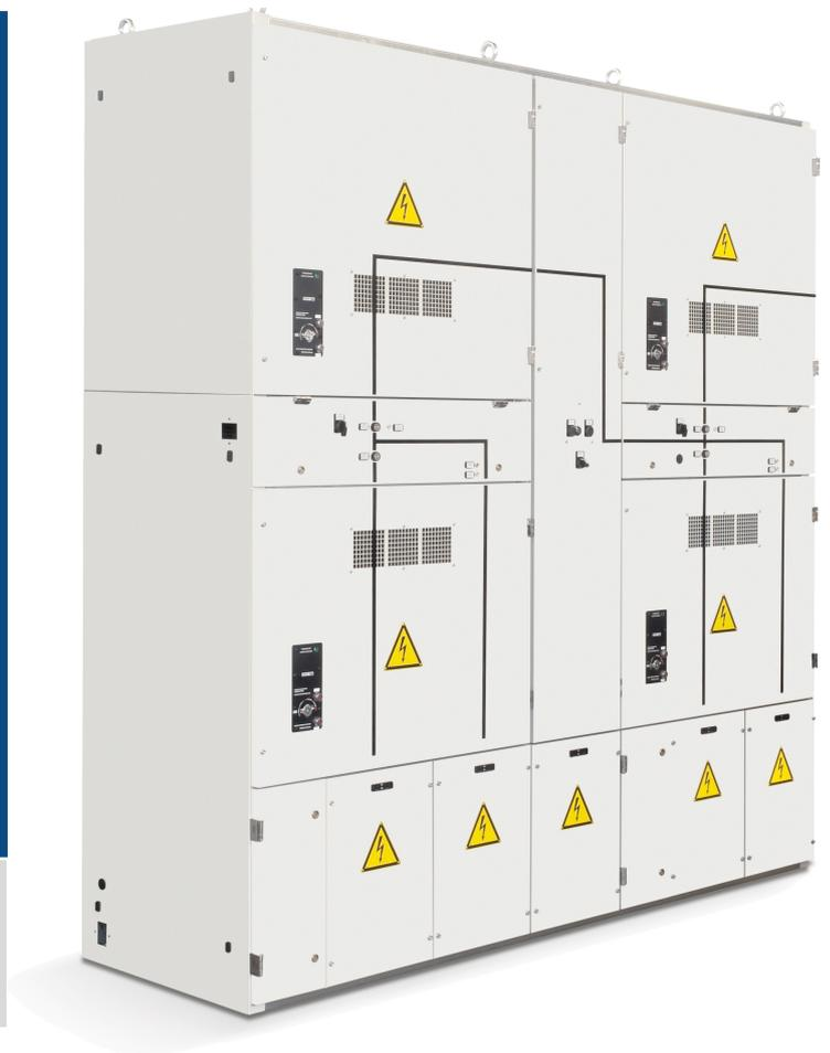
In DC Traction Substations one disconnector or load break switch is normally installed downstream each High Speed Circuit Breaker thus allowing, in case of failure, to isolate the circuit breaker granting the safety of the system. The configuration is then completed by a by-pass or parallel disconnector switch connecting two feeders and allowing to grant the service continuity in case of failure of one circuit breaker: this disconnector is normally on-load and motorised for remote control.
