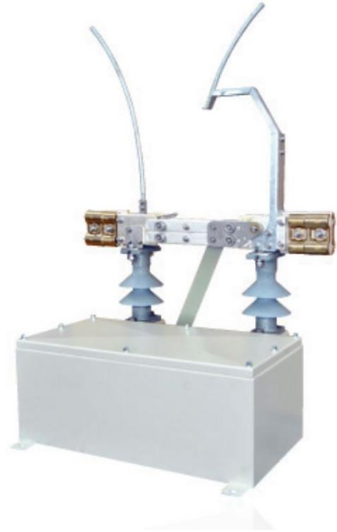
The Outdoor switch-disconnector SEC-1500 is suitable to be installed directly on the Overhead lines of TRAMWAYS and TROLLEYBUS systems with rated voltage up to 1500V. It is capable of making, carrying and breaking currents in normal and overload conditions.
