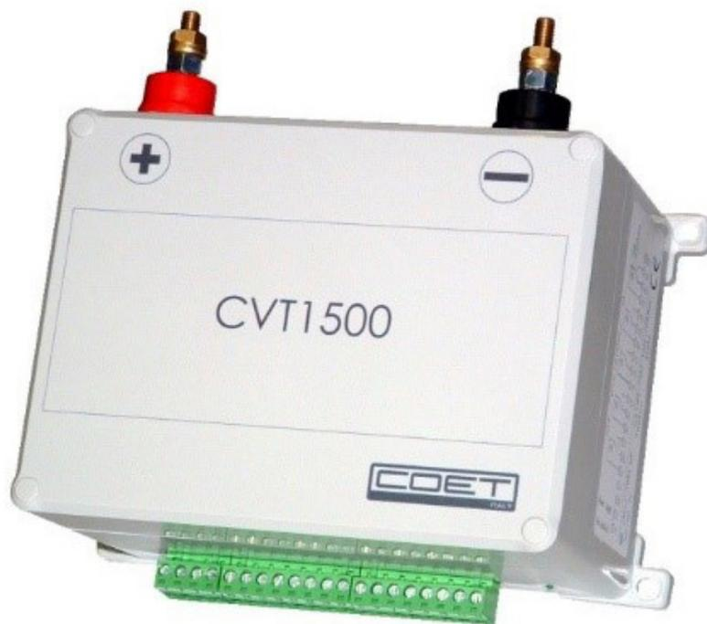
Voltage presence relay (F80) / undervoltage relay (F27) is normally used in dc circuits when the control of disconnectors or other safety devices must be locked in case the voltage is above a set value or the voltage absence on a line section must be signalized. It is used in all the Traction systems like tramways, trolley bus, Metro and Railways Power Supply Substations.
