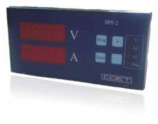
RPR-2 relay is the perfect solution for metering and Protection on traction rectifier. Used in combination with TIM Measuring Transducer guarantees the complete rectifier protection making also available Voltage, Current and Power (optional) measurements both locally (on the two 4 digits Led displays) and remotely via RS485 serial connection bus.
